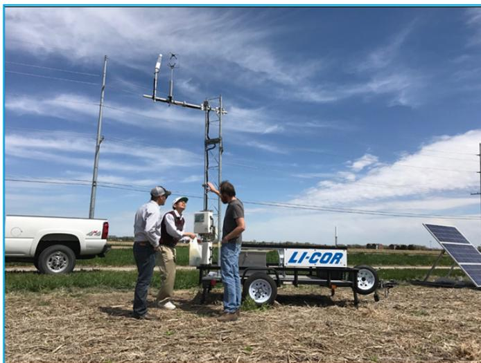
*The LI-COR Automated Evapotranspiration Station is located just south of West State Farm Road in North Platte, Nebraska, on the north end of the cornfield being monitored. This location was chosen because the prevailing summer winds are from the south. The analytical equipment is mounted approximately 12 feet above the ground, allowing it to measure crop activity within about 1000 feet of the station*
